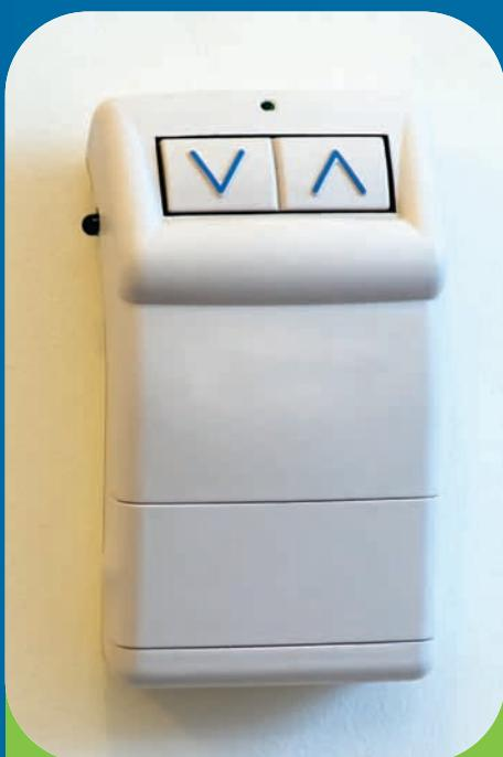
The wireless wall controls can be used to call the stairlift to you, or to send it to someone at the other end of the staircase.
